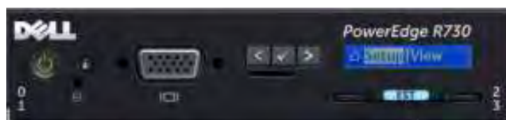
Figure 9. R730 LCD control panel
