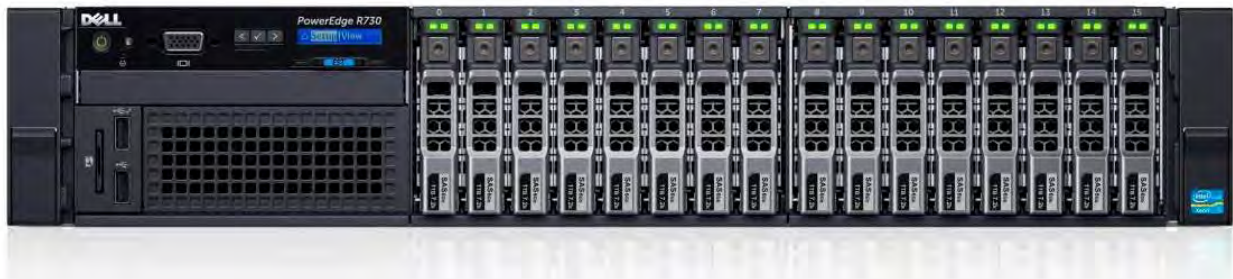
Figure 2. R730 front view (2.5" chassis without bezel)
