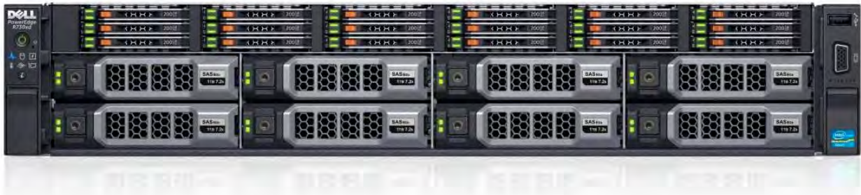
Figure 4. R730xd front view (8 x 3.5" plus 18 x 1.8" without bezel)
