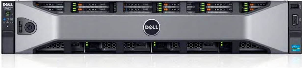
Figure 3. R730xd front view (8 x 3.5" plus 18 x 1.8" with bezel)
