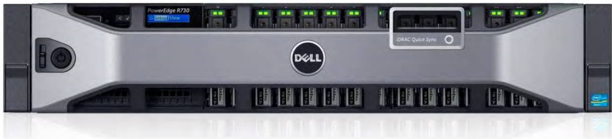
Figure 1. R730 front view (2.5" chassis with bezel)
